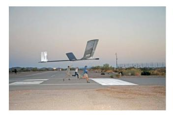
British defense company company QinetiQ says it has set the world record for unmanned flight with its <u>solar-powered plane Zephyr</u>, which flew for 82 hours 37 minutes, beating the current record of 30 hours 24 minutes set by American plane Global Hawk in 2001. Launched by hand, Zephyr is an ultra-lightweight, carbon-fibre, solar powered vehicle and is in industry parlance known as a high-altitude long-endurance (HALE) Unmanned Aerial Vehicle (UAV).
